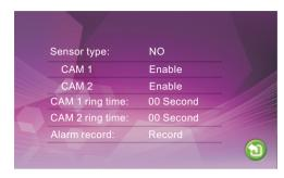
[Sensor type]: Each camera channel corresponds to an I/O status (see the following status explanations), which means that when an alarm is triggered, it will activate the corresponding channel to start alarm recording or capture a snapshot.
