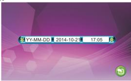
On system menu, move the cursor to "Time" and press "\*" to enter the "Time" menu. Use this field to switch the date format, include "YY-MM-DD" and "DD-MM-YY", to adjust system date and time. First scroll "" upward or downward to move the cursor, and press "\*" to select menu options, and then scroll "\*" upward or downward to adjust values, then press "\* again to confirm.
